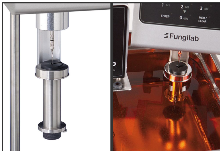
Fig. 4. Left picture: Assembled APM/B small volume adapter. Right picture: APM/B immersed in a thermostatic bath.
